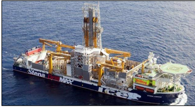
Figure 12 Floating Drillship Designed and Configured for Arctic Drilling (Source: Stena Drilling)
