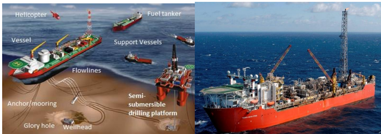
Figure 15: Schematic of Terra Nova (Source: Suncor) Figure 16: Terra Nova Floating Production, Storage and Offloading (Source: Suncor)
